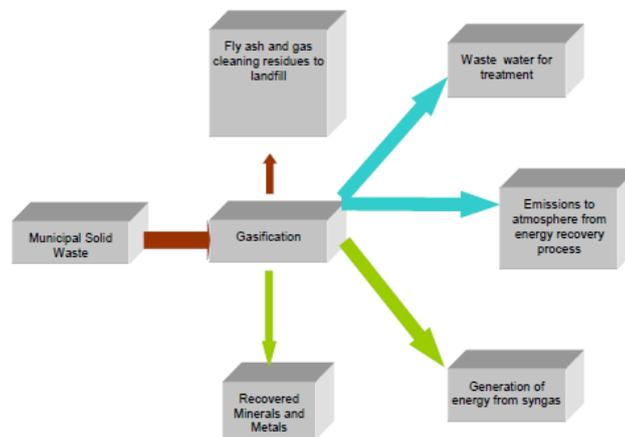
Figure 16. Schematic representation of gasification inputs and outputs
