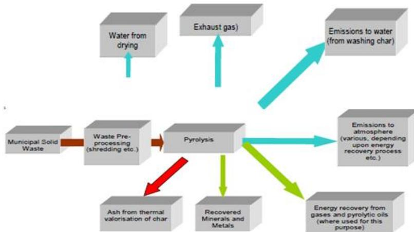
Figure 15. Schematic representation of single pyrolysis process inputs and outputs (Eunomia, 2015)
