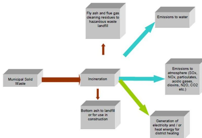
Figure 14. Schematic Representation of Incineration Inputs and Outputs (Eunomia, 2015)
